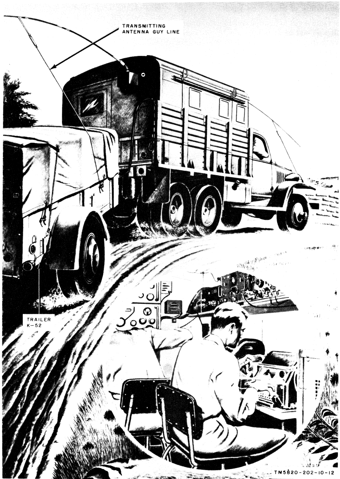
Figure 12. Radio Set AN/GRC-26(*) mounted on truck.
